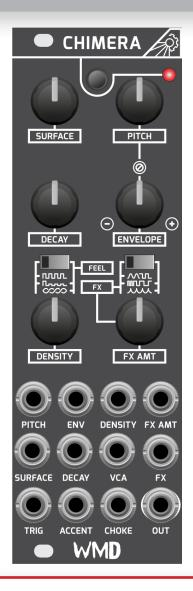
TRIG: Hit it with some pulses! For extra fun, trigger the module using the handy trigger BUTTON.
